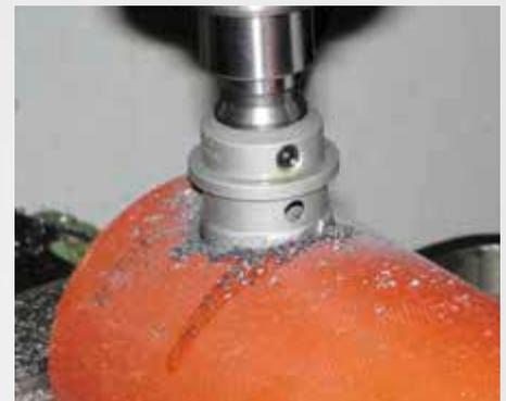
Bohren in Rohre
