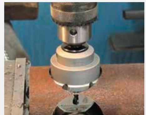
Bohren in Rohre
