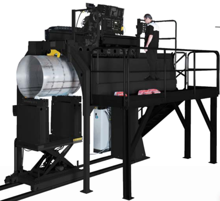
The Seamer benches for longitudinal weld of plates or vessels.
