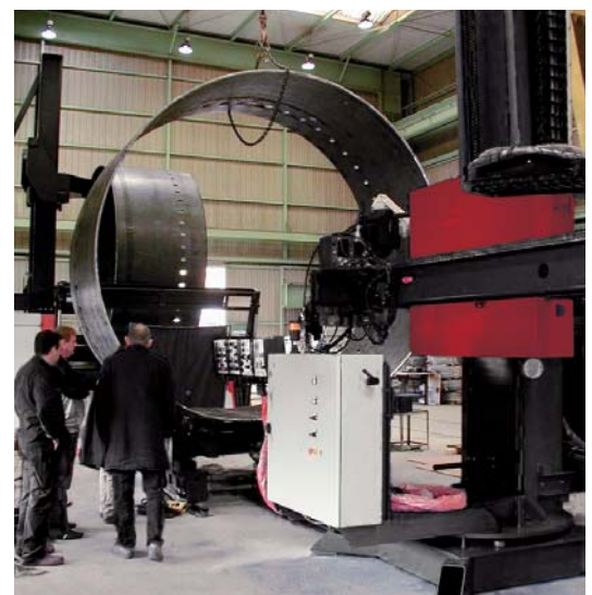
Large column and booms, rotators and positioners are proposed in this windmills solution.
