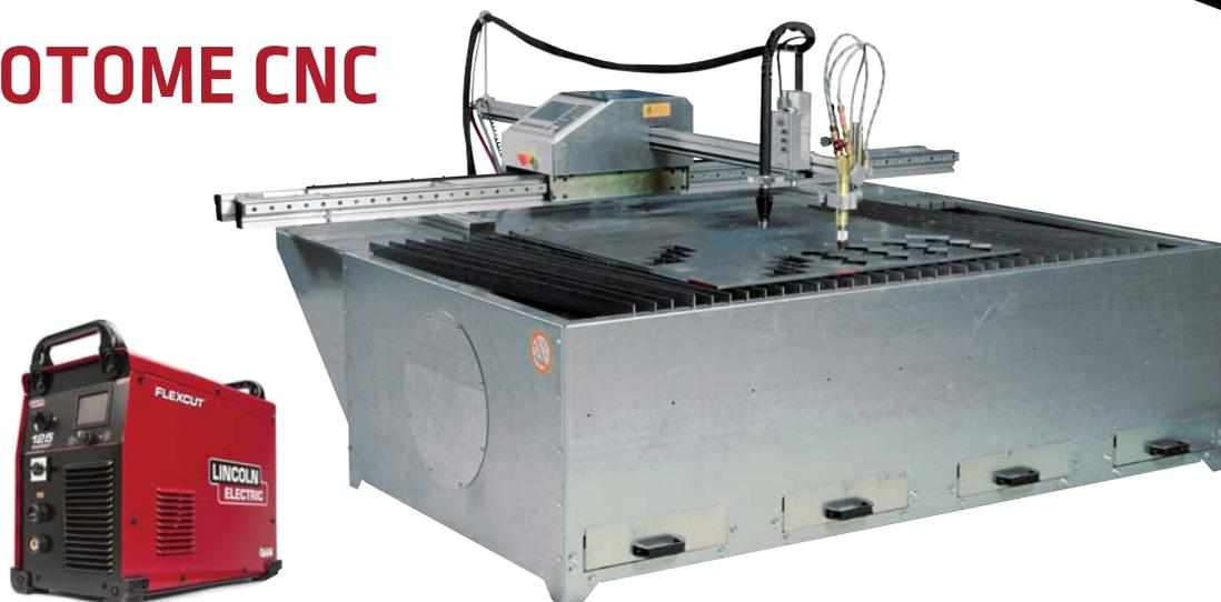
PYROTOME CNC is a small mechanised machine integrating a digital controller for cutting on metal sheets format of 1 000 x 2 000 mm or 1 500 x 3 000 mm. The programming is carried out from a library of standard shapes integrated in the digital controller or from the nesting software (in option). Equipped with one oxycutting torch or one plasma air installation, PYROTOME CNC is simple to implement, versatile, rugged and economical.
